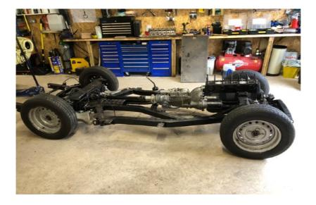
Dropped engine , gearbox and overdrive back on chassis. Draining gearbox of oil, bits of cog came with it. Removed gearbox and stripped down to find constant gear damaged and countershaft in poor shape, so decided to do a full refurb of gearbox. What a pain. I wouldn't do another, rather pay someone else and just get that pain.
